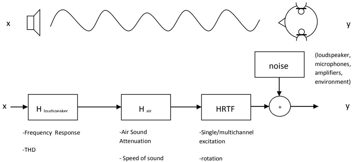
Figure 1. Transfer path model
